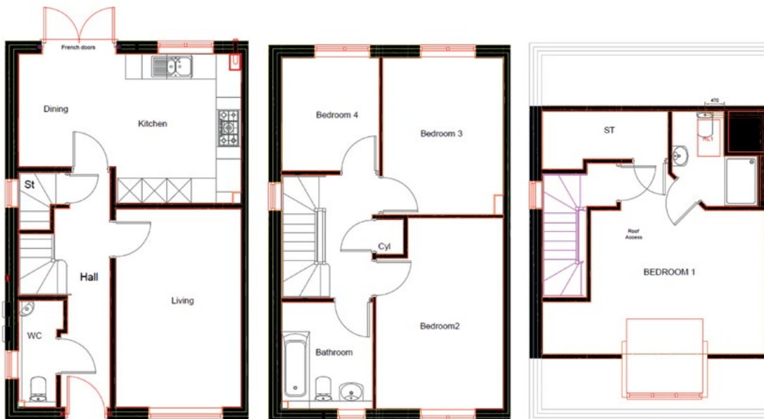
Figure 2: Semi-detached house type B floor plans (ground floor, first floor, mansard) – image courtesy of Woodall Homes
