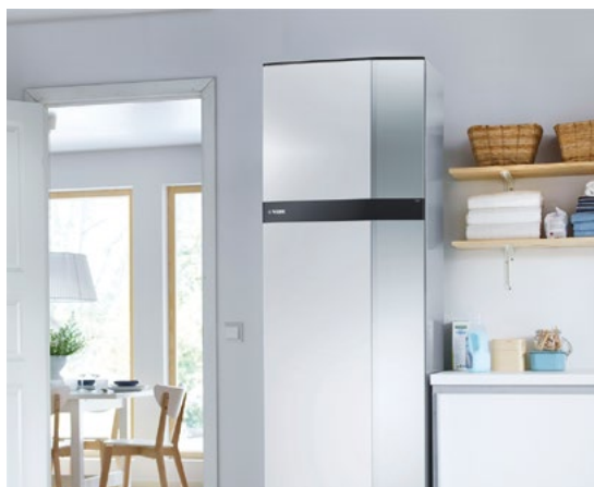
Figure 2: An example of an exhaust-air heat pump (EAHP) charged with R290 (propane) delivering heating, hot water and ventilation in one package, with a SCOP of 4.29 and a measured noise level of 49dB(A) (to EN12102). This is aimed at apartments and new-build houses up to 160m 2 (Source: NIBE)
