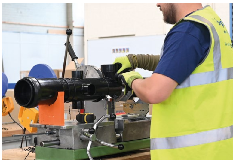
Figure 1: Offsite prefabrication of drainage systems in factory conditions allows for faster and more confident installation on site. Specialist fabricators and factory-controlled quality assurance systems (including pressure testing) ensure quality and reliability (Source: Polypipe Building Services)
